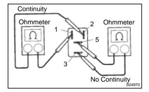
(c) Inspect the No. 1 cooling fan relay continuity.
